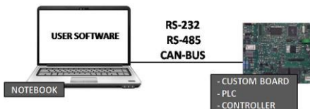
Figure B: example of local serial communication
