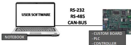
Figure B: example of local serial communication
